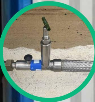
**Needle valve on transfer hose to limit cooling rate, reducing thermal shock**
