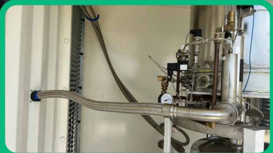
**Vacuum insulated pipework between test equipment and dewar**
