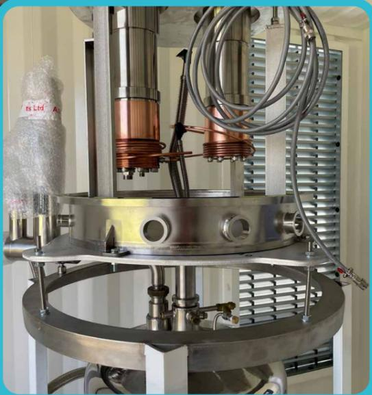
**Boil-off active management with two cold heads. Dewar ullage used to accommodate expansion and contraction of hydrogen, with constant pressure monitoring and control, via cycling between dormancy and reliquefaction of hydrogen gas**
