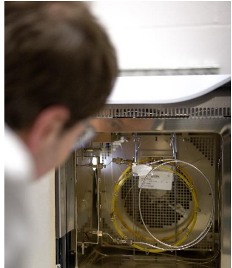
Figure 10 - Picture of Shimadzu GC-MS showing the Lead Chemist servicing the GC columns. The silver loop is a guard column to filter out gases harmful to the separation columns. The yellow and orange loops to the back of the oven are the GC separation columns providing light and heavy components.
