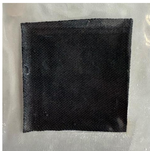
Bipolar Membrane – keeps both gases and electrolytes separate. Critical for separation of hydrogen and oxygen, whilst also preventing unwanted side reactions.
