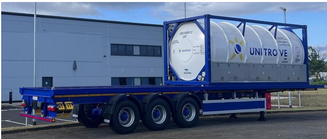
Figure 5 – Unitrove LH 2 Storage Tank
