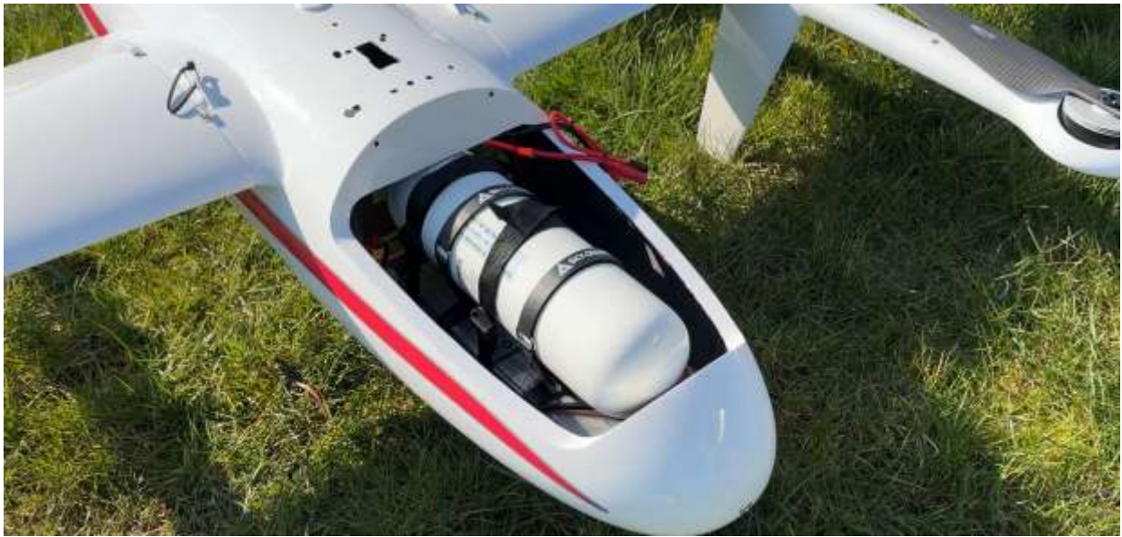
Figure 3.1: Hydrogen tank installation and securing mechanism
