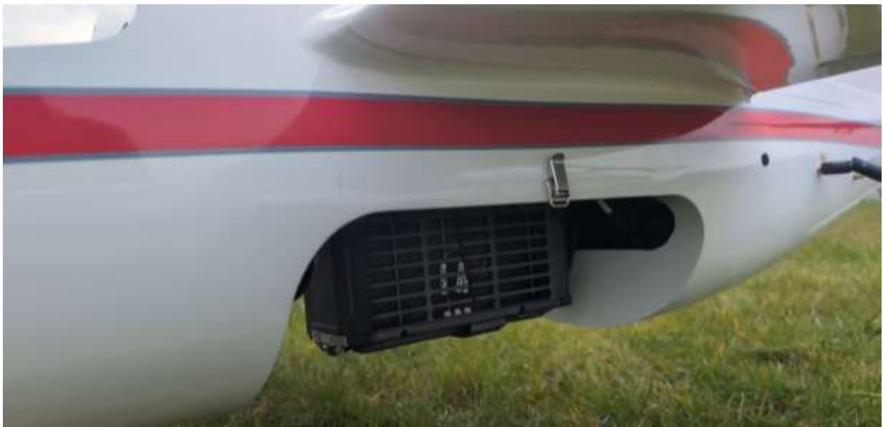
Figure 3.2: Fuel cell system installed within the UAV fuselage
