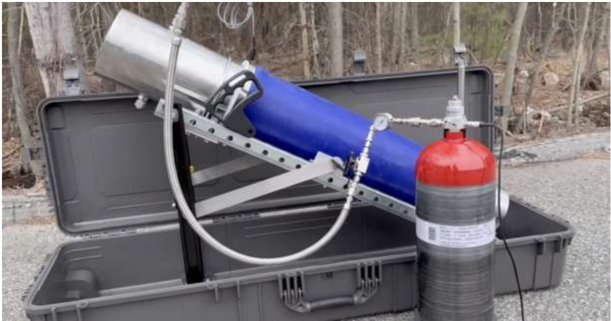
Figure 4.2.3: Tank Fueling by the Edge Refueler
