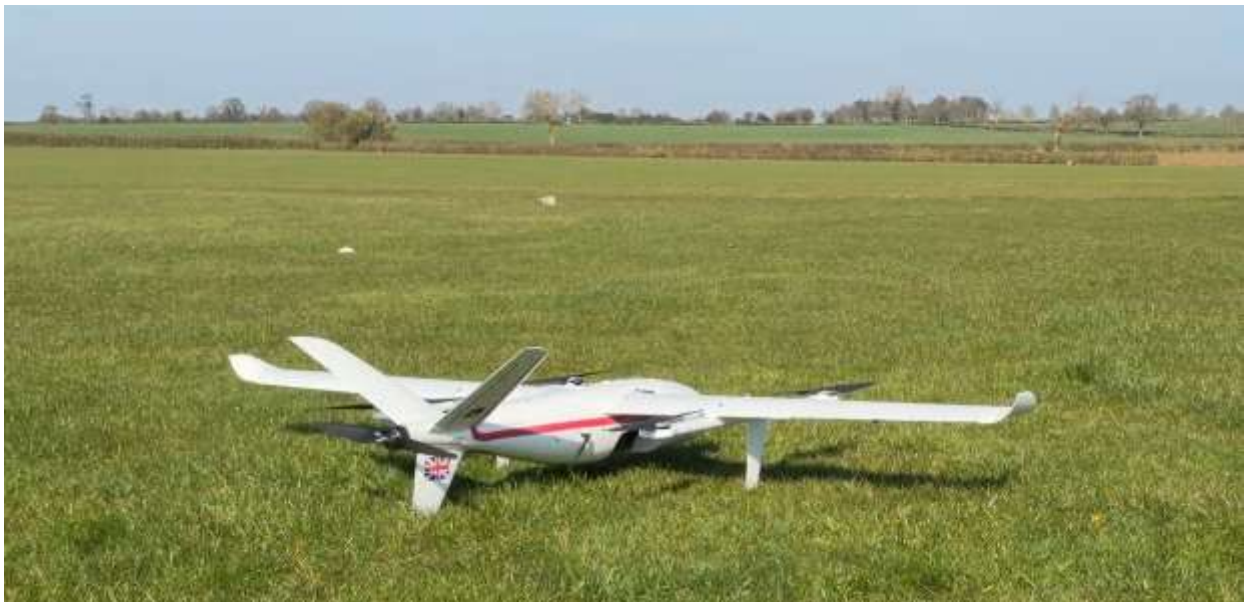
Figure 4.1.3: Hydrogen-powered UAV on the ground prior to flight testing
