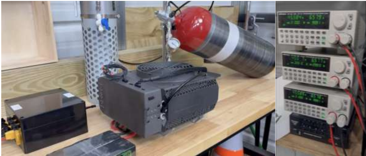
Figure 4.1.1: Hydrogen Tank and Fuel Cell Commissioning Test Setup
