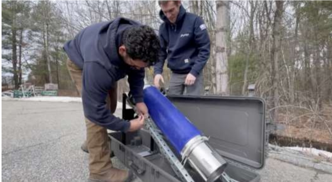
Figure 4.2.1: Setup of the Edge Refueler Hydrogen Generation System
