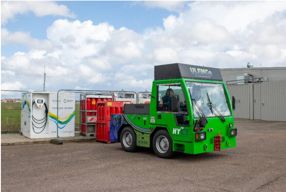
Figure 6 - Filling the MATT at Cranfield's Refueller
